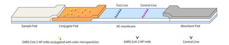
The COVID-19 Antigen Rapid Test is a lateral flow immunoassay based on the principle of the double-antibody sandwich technique. If the specimen contains SARS-CoV-2 antigen, a colored test line (T) would be visible in the result window. Absence of the T line suggests a negative result. The control line (C) is used for procedural control, and should always appear if the test procedure is performed properly.
